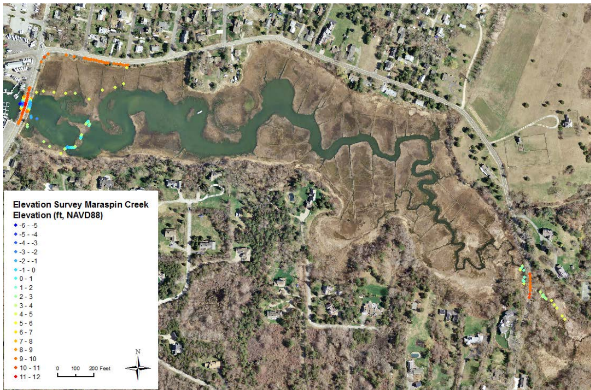
Figure 2: Maraspin Creek elevation survey of Millway Bridge, Maraspin Creek channel, and Commerce Road.
